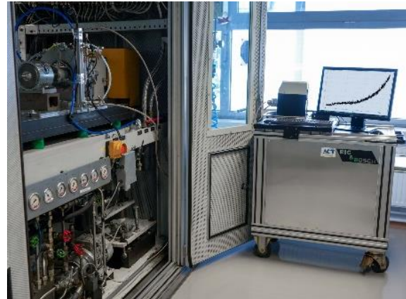
Left: Test bench with set-up of a transmission of the e-axle drive; Right: RIC measuring system with detected critical wear behaviour (Photo: AC2T research GmbH)
